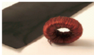
A replica of the first soft-ferrite core and a sample of ferrite-coated film for suppressing electromagnetic noise.
