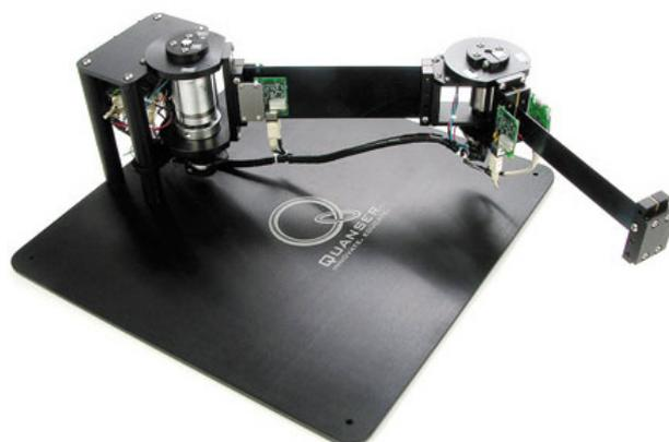
Fig. 6.11: The appearance of 2 DOF flexible link robot arm [55]
